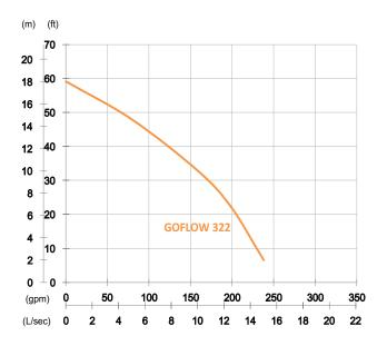
Shaft Speed: 3450 rpm Outlet: 80mm, 3in
